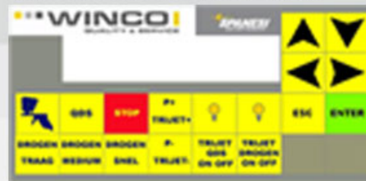
Cabine Manager SIEMENS TD200C
